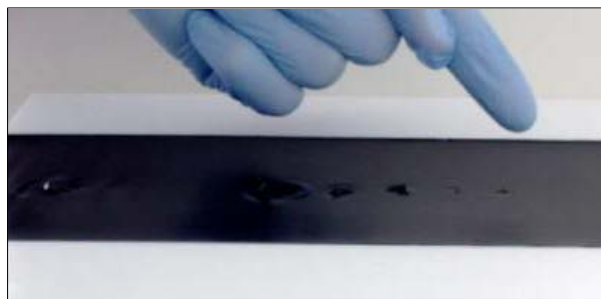
Figure 8: If no residues on your fingers are recognized the skin-over time has been reached
