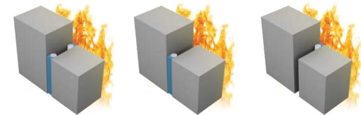
1. Double seal 2. Single seal, unexposed side 3. Single seal, exposed side
