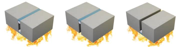
1. Double seal 2. Single seal, unexposed side 3. Single seal, exposed side
